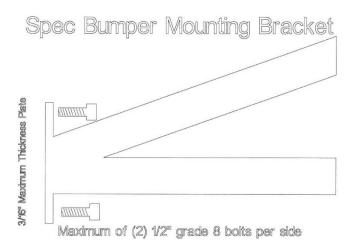
(1)Bracket per side of the car. Wrap around bars may circle around and be welded to the frame horn. No other bracing is allowed. Mounting bracket must also be made of 1 ½" x .095 round tubing
