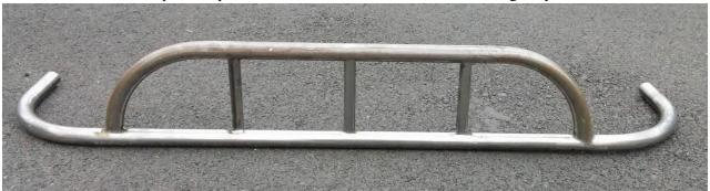
We will be allowing diagonal braces as pictured below on the mounting plates AND (2) more bars made out of 1" x .095 round tubing. These 1" bars may be used as kickers to the core support or the frame horns. They cannot extend rearward past the factory core support location.
