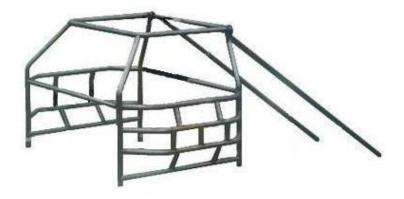
Door bars and overhead welds must be gusseted.
