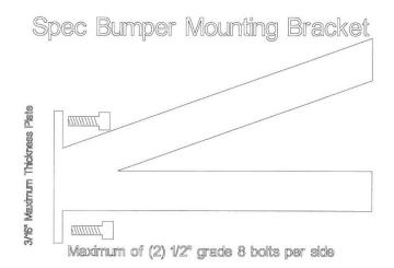
(1)Bracket per side of the car. Wrap around bars may circle around and be welded to the frame horn. No other bracing is allowed. Mounting bracket must also be made of  $1 \frac{1}{2}$ " x .095 round tubing
