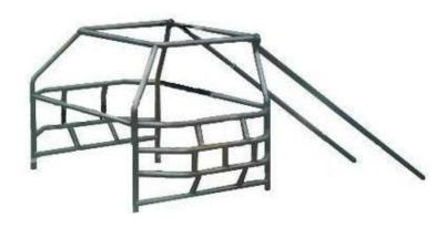
Door bars and overhead welds must be gusseted.
