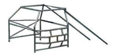
Door bars, passenger side "X" and overhead welds must be gusseted.
